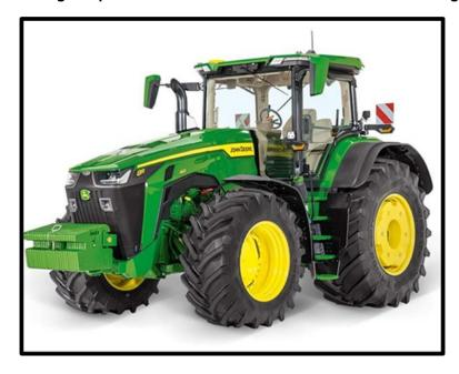
The new tractor pulls a 42-foot airfield mower and is utilized by Airport Maintenance for airfield mowing. The new tractor/mower performs the work of three (3) existing mowers.
